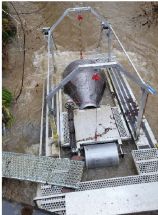
Little River screw trap during a high flow event. The water is supposed to flow under the pontoons!
